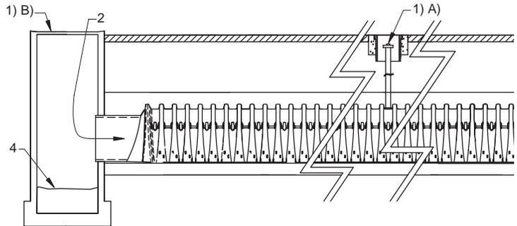
**Step 2)** Clean out Isolator Row using the JetVac process
